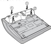
To attach the wall mounting adaptor, push it in the direction of the arrows (1) and (2) as shown.
