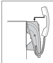
To temporarily set the handset down during a conversation, place it as shown here.
